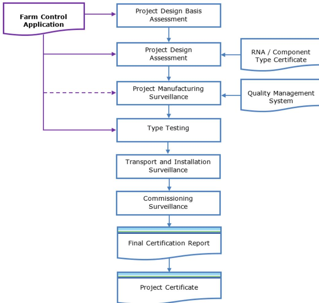
Figure 5 Modular structure of project certification as per DNV GL service specification
