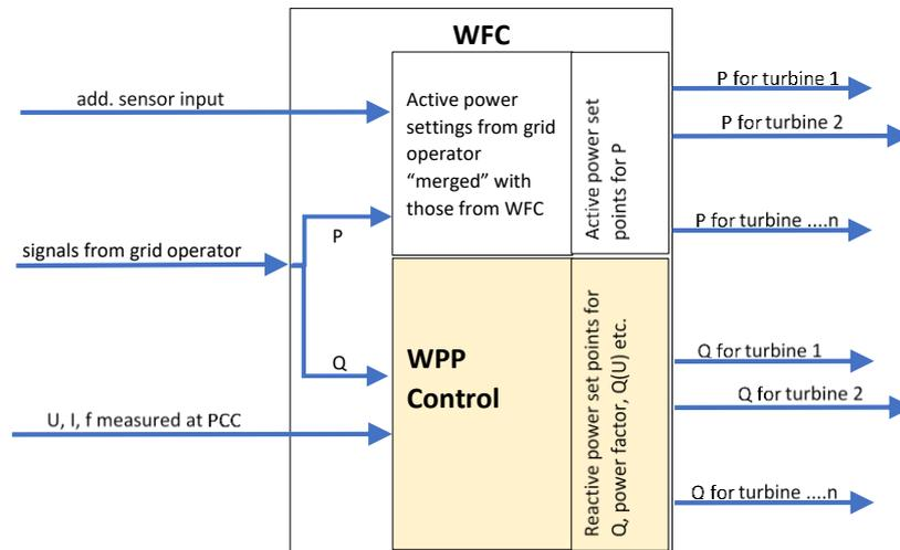
Figure 27 Integrated approach for co-ordination between WPP control and WFC
