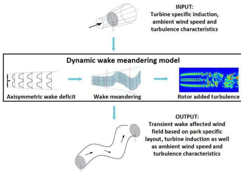
Figure 25: Dynamic wake meandering model based on velocity deficit according to Ainslie's model
