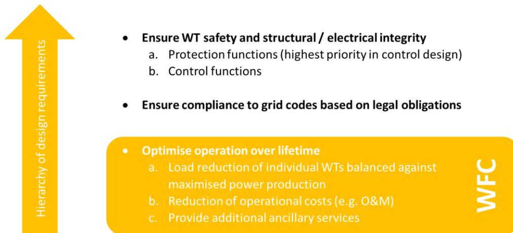
Figure 9 Hierarchy of design requirements applying WFC from certification's perspective
