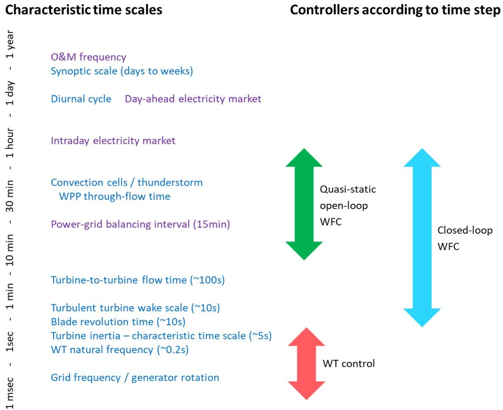
Figure 10 Characteristic time scales for control tasks (based on Total Control [17])
