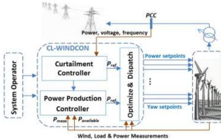
Figure 8 Proposed control scheme for WFC as proposed in CL-Windcon EU project
