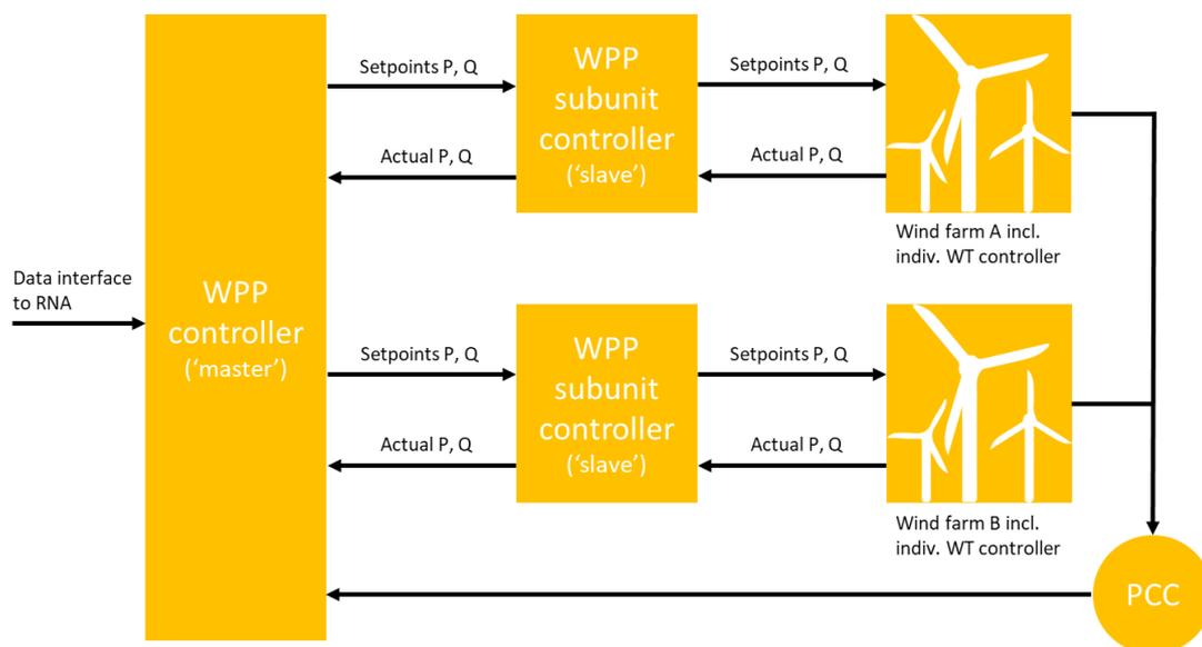
Figure 7 Arrangement of WPP sub-unit and common controllers in mixed wind farms
