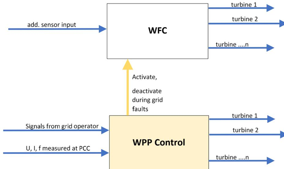
Figure 26 Parallel approach for co-ordination between WPP control and WFC
