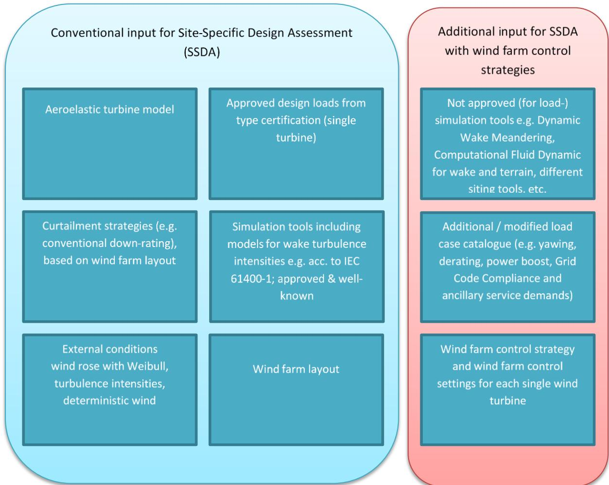
Figure 29 Conventional Site-Specific Design Assessment (left) and additional input for wind farm control strategies (right)
