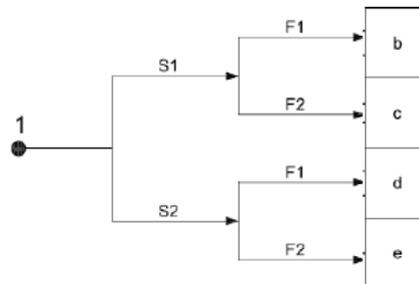
Figure 30 Risk graph for determining protection functions PLr as per ISO 13849-1
