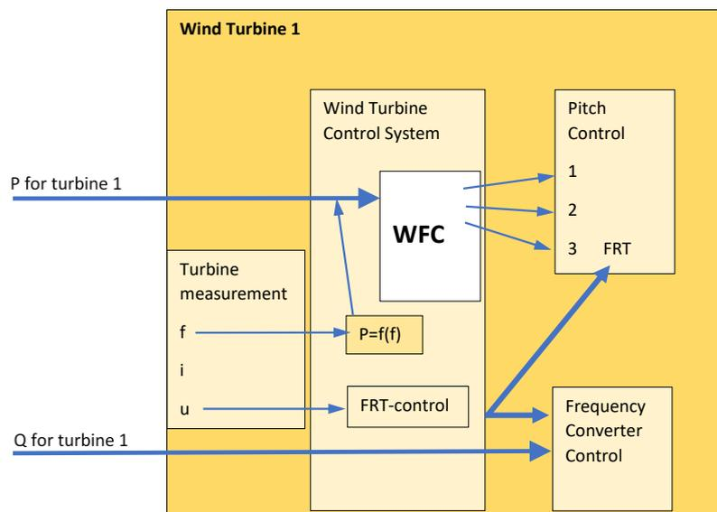
Figure 28 Additional co-ordination of WPP control and WFC on wind turbine level
