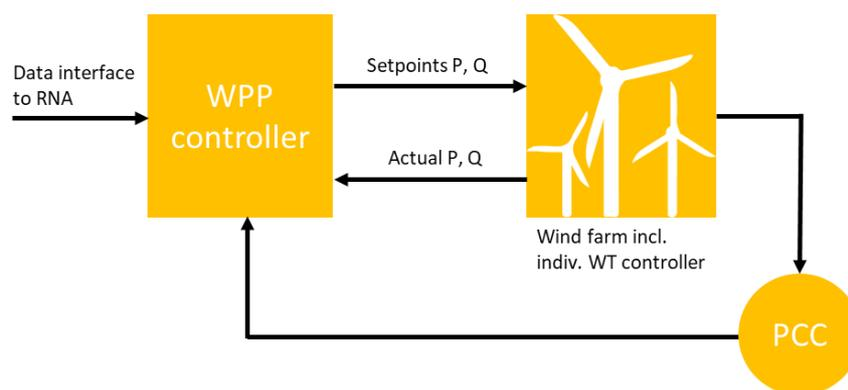
Figure 6 Standard arrangement of the WPP control unit in a wind farm without WFC
