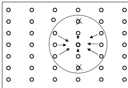
Figure 24: Configuration inside a wind farm with more than 2 rows, Annex E [84]
