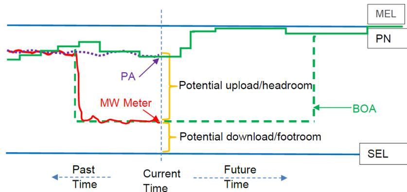
Figure 22 PA signal and WPP module frequency support during BM window(NationalgridESO)
